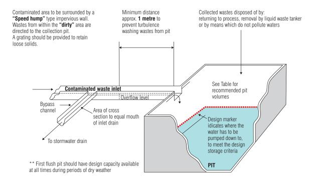
This diagram is for illustrative purposes only and each First Flush system should be specifically designed to meet all applicable State regulations, site requirements and weather conditions.
